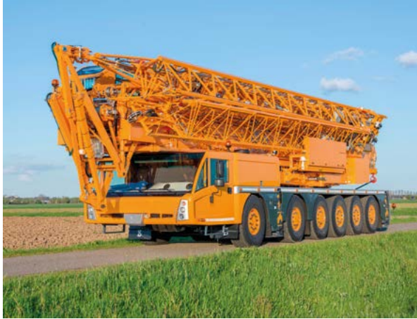
Electric cranes are on the upswing: Crane manufacturers are increasingly relying on cranes with fully electric lifting systems such as this six-axle mobile tower crane. Crane models with electric systems for both lifting and driving are also already available. ( www.spieringscranes.com )
