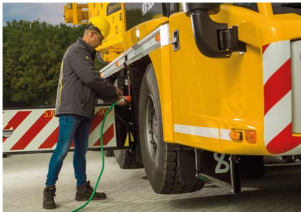
Plugged in: Electric construction equipment can be charged via AC or DC charging stations.
