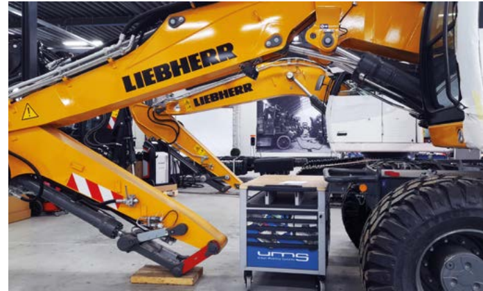
Ready to be retrofitted: Brand-new common construction machines are fitted with electric drive systems by specialist retrofitters. ( www.urbanmobilitysystems.nl/en )
